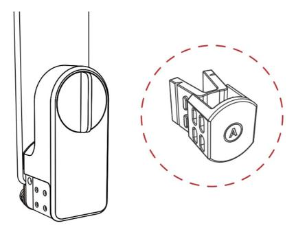
**B8.** Short knob: Open the knob of the main body, push out the Clamp A, insert the Clamp B, and then put the knob back to its original positioning.
