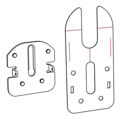
3. Align the center of the knob with the crossed red line, attach the mounting plate to the door, and remove the card.
