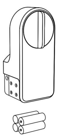
**A6.** Install the main body on the mounting plate.
