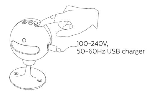
**NOTE:** When the host broadcasts the voice, even you triggers any button on the host, the host state does not change.
