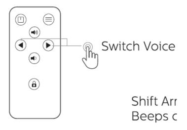
Shift Arm and Disarm, Beeps once means Arm, Beeps twice means Disarm.
