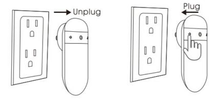
Press and hold (don't release it), plug in the receiver.
