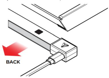
5. Align the end of the strip with the side of the desk and magnetically attach the end connector to the underside of the desk.
