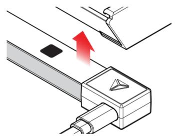
6. Attach the remaining length of the Secretlab MAGRGB™ strip to the underside of the desk, making sure that each of the embedded magnets snaps into place.
