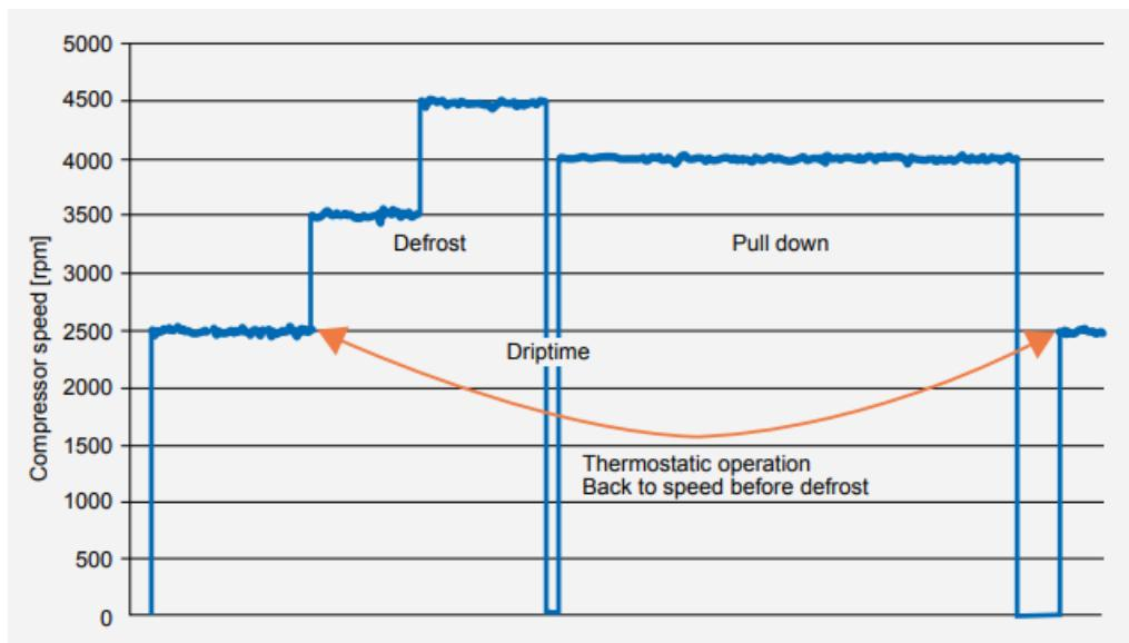
When variable-speed compressors are used in self-adapting capacity modes, defrosting may not work properly since the compressor speed cannot be controlled during defrost: The compressor lacks capacity for hot gas and the following pull-down.
