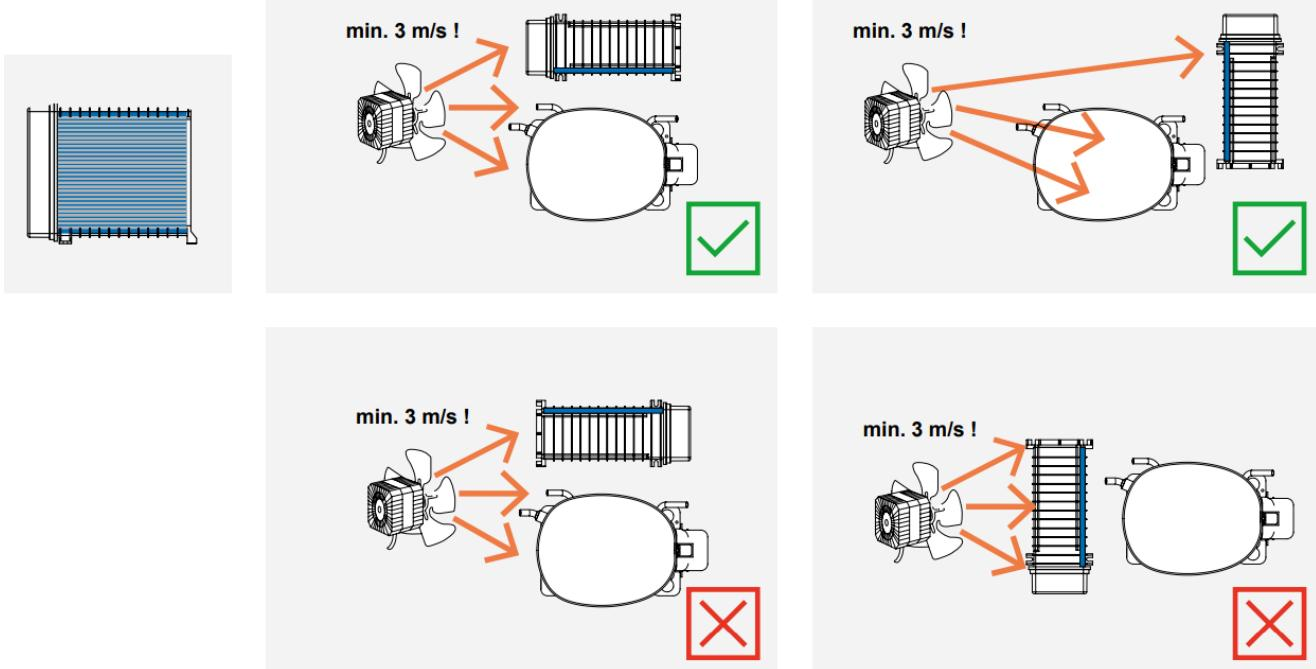
Ensure proper airflow of 3 m/s at both compressor and electronic units.
