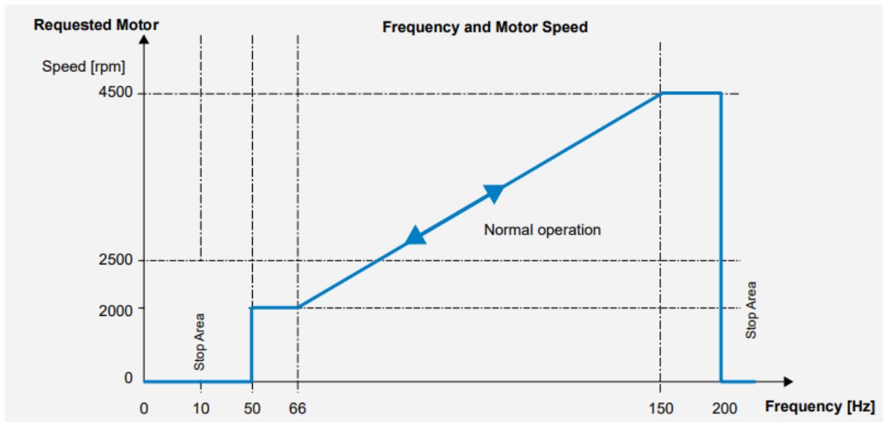
The speed can be controlled by applying a low voltage frequency signal to the frequency input
