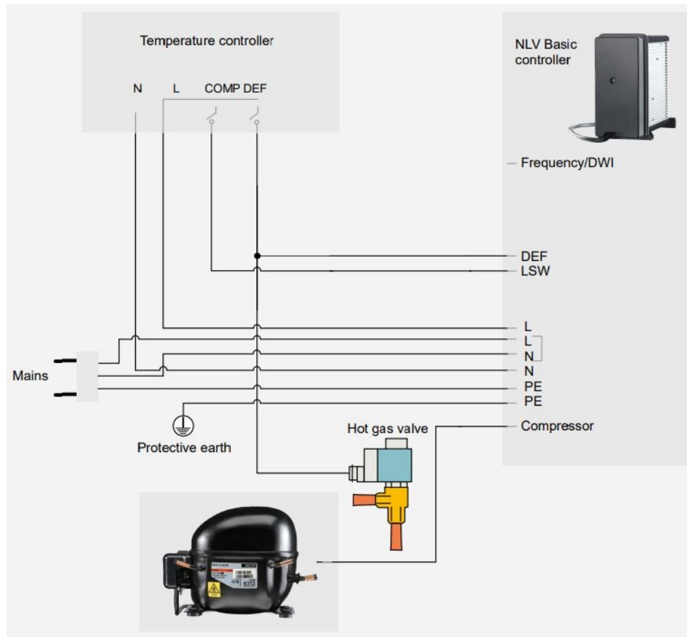
For optimal hot-gas defrost performance, the relay output of the controller should be connected to the DEF input of the controller.
