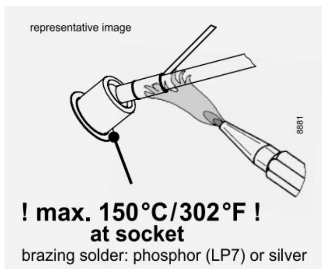
Refer to Product Bulletin: Brazing on Suction Connectors (Compressors with Direct Suction Intake)
