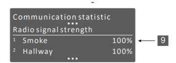
Radio signal strength in a wireless environment indicates how well the control panel or module can "hear" a signal from the detector 9.
