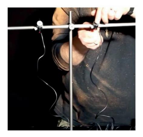
With the double cross laser, the height is adjusted via the fixed joint, which serves as an intermediate element between the vertical and horizontal rods. Tighten the knurled screw on the vertical rod only after the desired height has been reached.
