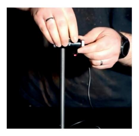
The height is also adjusted using this joint. With the single cross laser, this can be done very easily by loosening the knurled screw on the side of the rod until the desired height is reached and then tightening it hand-tight.
