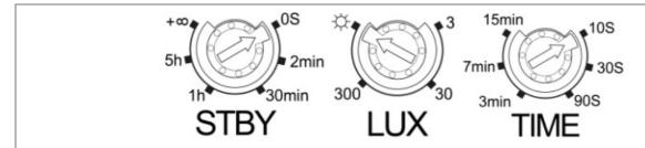
Ensure that the motion detector is not obscured. Ensure that the coverage area is not restricted by items such a s through large furniture. To set the detection range and the daylight test, turn the knobs to the positions shown. The motion detector is activated after a warm-up phase of approx. 30s. If no further movement takes place in the sensing area of the sensor, the sensor switches off.
