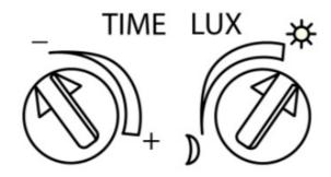
Ensure that the motion detector is not obscured. Ensure that the coverage area is not restricted by items such as through large furniture. To set the detection range and the daylight test, turn the knobs to the positions shown. The motion detector is activated after a warm-up phase of approx. 30s. If no further movement takes place in the sensing
