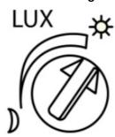
This setting control can be used to regulate the switch-on sensitivity of this unit depending on the ambient brightness (between 3 and 2.000 LUX).
