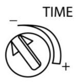
The duration of the operating time can be set continuously from approx. 10s to 5min. The timer is restarted if a movement from the sensor is detected before the set time has elapsed.
