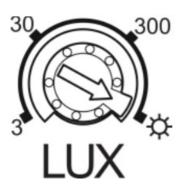
This setting control can be used to regulate the switch-on sensitivity of this unit depending on the ambient brightness (between 3 and 2.000 LUX)
