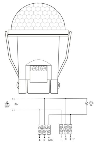
Permanent switch-on of a connected device with an additional switch connected in parallel (see Fig.4b).
