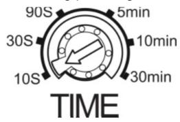
The duration of the operating time can be set continuously from approx. 10s to 30min. The timer is restarted if a movement from the sensor is detected before the set time has elapsed.
