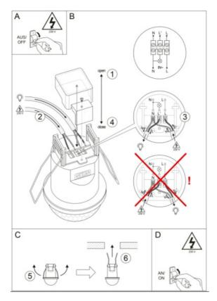
**Danger:** Before installing please make sure that the circuit is interrupted! For installation, the work on the mains voltage is required. Please remove the associated mains fuse or deactivate the switch fuse! Check by using a voltage tester if the line is de-energized. Make sure that the current circuit will not closed during the installation!
