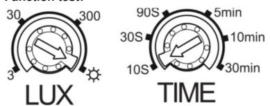
Ensure that the motion detector is not obscured. Ensure that the coverage area is not restricted by items such as through large furniture. To set the detection range and the daylight test, turn the knobs to the positions shown. The motion detector is activated after a warm-up phase of approx. 30s. If no further movement takes place in the sensing area of the sensor, the sensor switches off.
