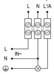
When connecting a lamp with protective conductor contact, the protective conductor must be bypassed from the supply line to the lamp with the aid of an additional terminal in the in-wall socket
