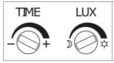
Ensure that the motion detector is not obscured. Ensure that the coverage area is not restricted by items such as through large furniture. To set the de tection range and the daylight test, turn the knobs to the positions shown. The motion detector is activated after a warm-up phase of approx. 30s. If n o further movement takes place in the sensing area of the sensor, the sens or switches off.
