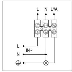
When connecting a lamp with protective conductor contact, the protective conductor must be bypassed from the supply line to the lamp with the aid of an additional terminal in the in-wall socket.
