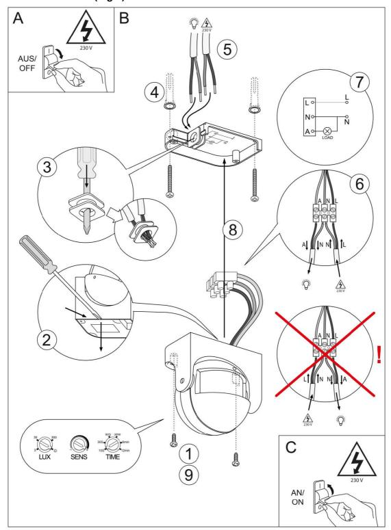
**Danger:** Before installing please make sure that the circuit is interrupted! For installation, the work on the mains voltage is required. Please remove the associated mains fuse or deactivate the switch fuse! Check by using a voltage tester if the line is de-energized. Make sure that the current circuit will not closed during the installation! **Danger:** The installation of this product may be done only by a qualified person according the valid regulations for electrical installation!
