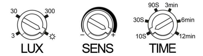
To set the detection range and the daylight test, turn the knobs to the positions shown. The motion detector is activated after a warm-up phase of approx. 30s. If no further movement takes place in the sensing area of the sensor, the sensor switches off.
