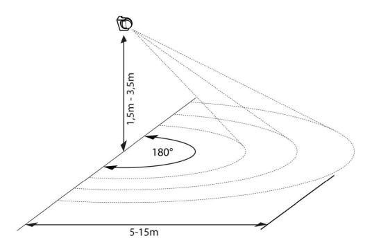
The detection range of the motion detector is approx. 5-15m and 180° (free area) at a mounting height of 1,5-3,5m on the wall. In closed rooms the detection distance can be lower, according to room layout.
