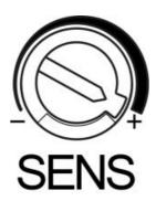
With this setting controller, the detection range of approx. 5m to 15m can be set. Turning the adjuster to the left will extend the range.
