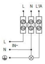
If a lamp with protective earth contact is connected and a junction box is not installed, the protective earth must be bridged from the supply line to the lamp by means of an additional terminal in the housing of the motion detector.
