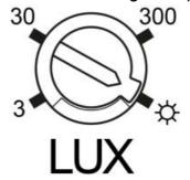
This setting control can be used to regulate the switch-on sensitivity of this unit depending on the ambient
