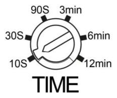
The duration of the operating time can be set continuously from approx. 10s to 12min. The timer is restarted if a movement from the sensor is detected before the set time has elapsed.
