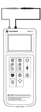
**Note:** A maximum test lead resistance of  $10\Omega$  ohms can be taken into account. If the test lead resistance is greater than  $10\Omega$  an error beep will indicate that the lead Zero function has failed.
