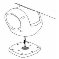
7. Using your own hardware secure the open array radar to the adapter plate. (Refer to the radar manufacturer installation instructions)
