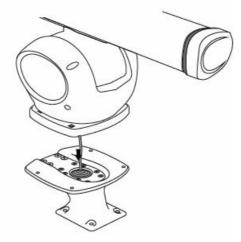
9. Secure the assembly using the four 3/8" x 1 1/2" bolts and washers.
