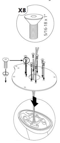
7. Apply marine adhesive sealant to the circular groove on the underside of the adapter plate. Then place the adapter plate onto the lower adapter plate. Make sure that the bolt holes line up.
