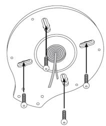
5. Attach the satellite dome to the adapter plate, and secure it with the hardware for your electronics.
