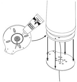
8. Secure the two adapter plates together with the four  $1/4-20\times1$ " bolts and nylon shoulder washers.
