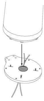
6. Attach the lower adapter plate to the Seaview mount with the eight 5/16-18 x 1" bolts and nylon washers.
