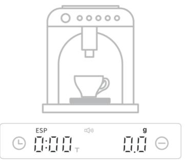
Turn on the espresso machine. When the coffee drops into the cup, the coffee scale starts to calculate the weight and automatically counts. After the drip is over, the timing and weighing stop. Take away the cup, and the coffee scale will return to the initial state for the next brew.
