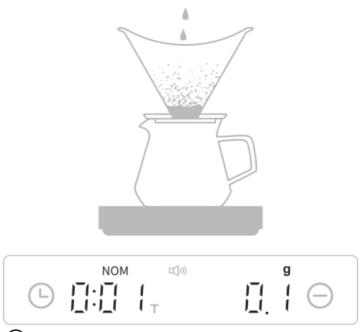
After brewing, press the "  $\bigcirc$  " timing key briefly to stop the timing, and the coffee scale will accurately display the brewing data for you.
