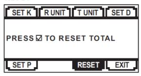
Reset the total flow volume to zero. This tab is not available when the -64 non resettable total option is ordered
