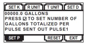
The factory setting will show Set P which allows one to view or change the volume of flow totalized per pulse sent to pulse out 1. The units for Set P follow the units selected for the rate display. (With EXIT highlighted, pressing the up arrow four times will access the secondary menu. The P/A tab in the secondary menu will allow pulse out 1 to be an alarm. The alarm can be set to trigger on either a high or low flow condition as determined by the user.)
