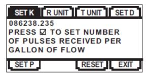
View or change the K factor. The K factor is the number of pulses the flow sensor provides for every gallon of flow. (Note that the decimal is fixed at three places. If you only have two decimal places for your K-factor, enter a zero for the third digit. If unable to set K-factor, the unit is "locked" to prevent tampering. Please contact your distributor for assistance.)
