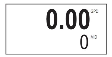
The HOME Screen, shown above, is the normal screen which displays TOTAL flow volume and flow RATE. The Four buttons below the LCD display are used to access menu screens for viewing and changing setup parameters.
