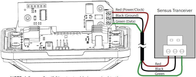
**NOTE:** A Sensus 2m (6 ft) output cable is prewired to the Seametrics product at the factory. Longer cables are optional.
