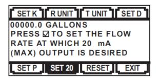
Input the flow rate at which 20 mA (max) output is desired
