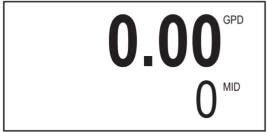
The HOME Screen, shown above, is the normal screen which displays TOTAL flow volume and flow RATE. The Four buttons below the LCD display are used to access menu screens for viewing and changing setup parameters. **Menu Navigation**
