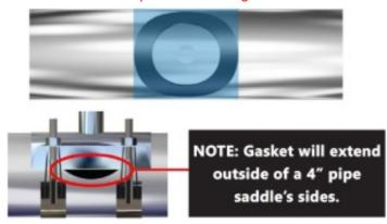
4. Place the saddle clamps under the pipe and align with the clamp guides on the saddle top.
