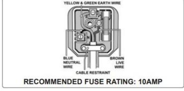
• Double insulated products, which are always marked with this symbol, are fitted with live (brown) and neutral (blue) wires only. To rewire, connect the wires as indicated in diagram.
