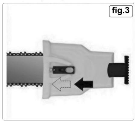
4. Run chainsaw whilst gently squeezing the chainsaw sharpener down until the teeth touch the whetstone for 3 to 5 seconds.
