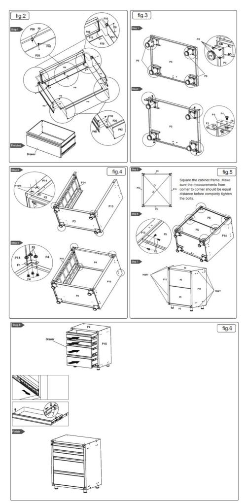
To place the draw back, simply push the ball bearing carriage all the way to the endof the slides (on both sides), and align the side runners on the drawer with the sidetracks on the unit. Push it carefully until it stops.
