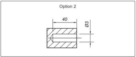
**Step 10.** To fix the cabinet to a wooden wall drill a hole using the illustration in option 2 as a guide.
