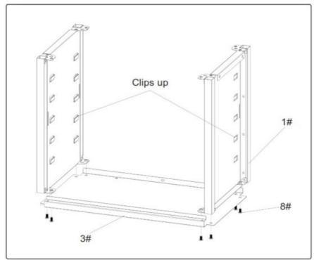
Step 1. Assemble the side panels, attach bottom panel with screws M6\*12 as shown.
