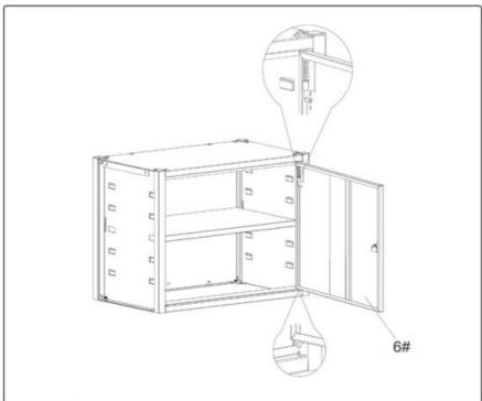
Step 6. Assemble the door as shown.
