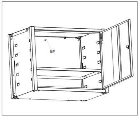
Step 9. Fix the cabinet to the wall using self-tapping screwST4.8\*30.
