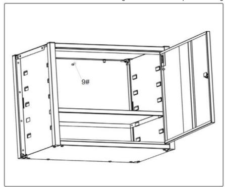
**Step 11.** Fix the cabinet to the wooden wall with the self-tapping screw ST4.8\*30, no expansion plug is required.
