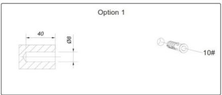
**Step 8.** To fix the cabinet to the wall, mark the wall out before drilling the hole, drill the hole and insert the expansion plug.
