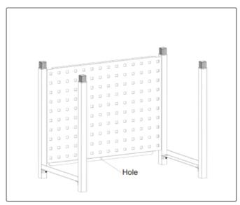
• Step 4. To fix the cabinet on the wall. Mark the wall out before drilling the hole, after the wall has been marked out drill a hole the size required see above illustration, insert the wall plug 8\*40 into the drilled hole.
