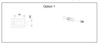
• Step 5. Fix the cabinet to the wall using the self-tapping screw ST4.8\*30.
