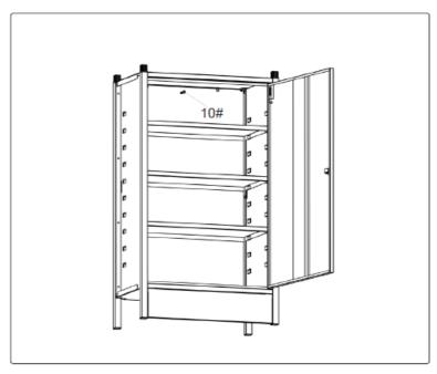
10. Step 10. Fix to the wall using self-tapping screw ST4.8\*30.
