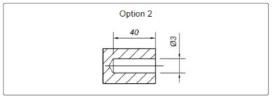
11. Step 11. To fix the cabinet on to a wooden wall. Mark the wall before drilling. After the wall has been marked, drill a hole the correct size using the size guide in the above illustration.
