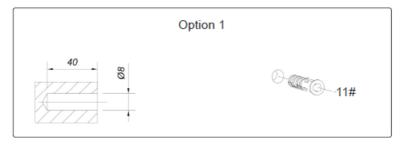
9. Step 9. After marking the wall. Drill a hole the size required, see the illustration. Insert wall plug 8\*40.
