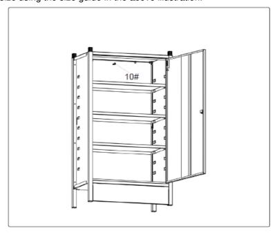
12. Step 12. Fix to the wall using self-tapping screw ST4.8\*30. Wall plug not required.
