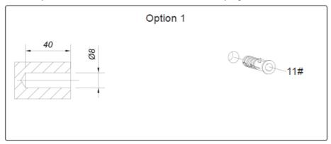
• Step 7. Fix cabinet to the wall using self-tapping screw ST4.8\*30.
