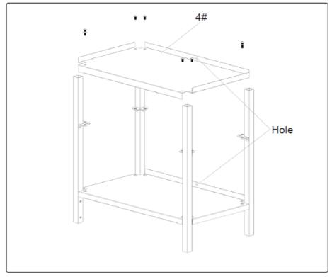
• Step 3. Assemble the skirting board to the uprights using screws M4\*10.
