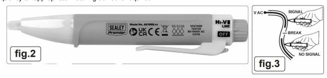
3. Insulated cores may be checked for continuity breaks (fig.3).
