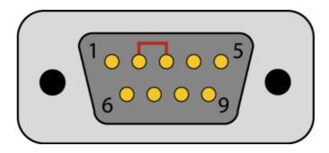
• RS-422 requires pins 1 & 4 (Receive + and Transmit +) and also pins 2 & 3 (Receive – and Transmit -) to be jumpered as shown in this graphic:
