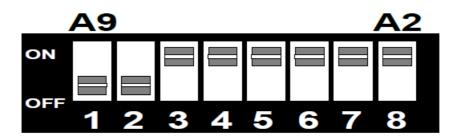
Setting the switch 'On' or 'Closed' corresponds to a '0' in the address, while leaving it 'Off' or 'Open' corresponds to a '1'.
