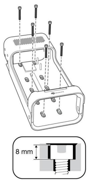
To avoid damaging Lyve Mobile Array's enclosure, the cylindrical socket cap on the mounting screws cannot
