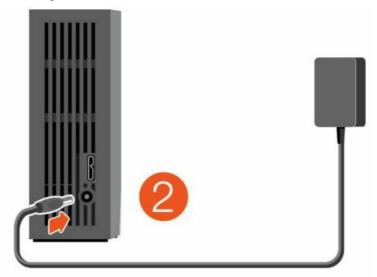
3. Connect the power supply to a live power outlet
