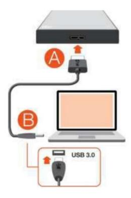
You can connect your Seagate device to a USB-C port on your computer. The USB-C port must support USB 3.0 or higher. A USB micro-B to USB-C cable is not included with this device.
