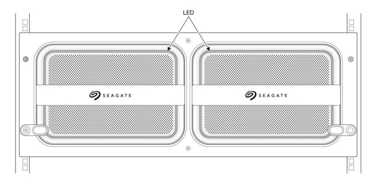
Once the device has been unlocked by a valid Lyve Portal Identity or Lyve Token file, the LED on the device turns solid green. The device is unlocked and ready for use.
