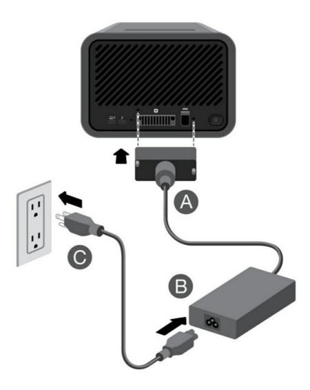
Use only the power supply provided with your device. Power supplies from other Seagate and third-party devices can damage Lyve Mobile Array.
