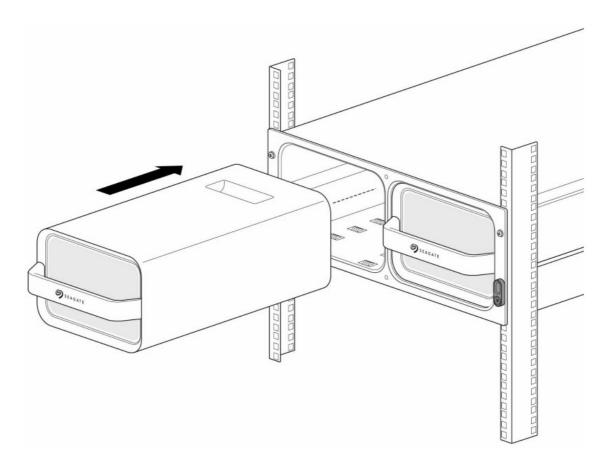
Slide device in until it's fully inserted and firmly connected to Rackmount Receiver's data and power. Close latches.
