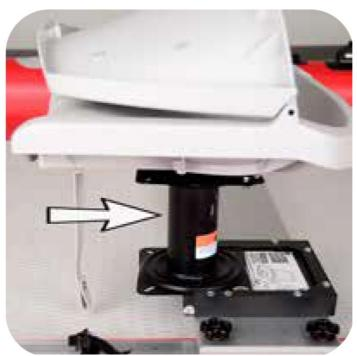
• To swivel the seat, pull locking bar forward then turn the seat.
