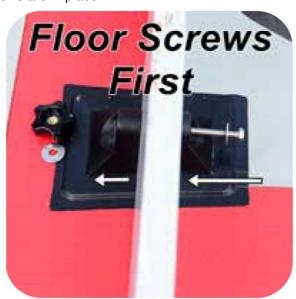
• A phillips head screwdriver is helpful for lining up holes. Also, push and pull the transom fore and aft to help the screws through the holes.
