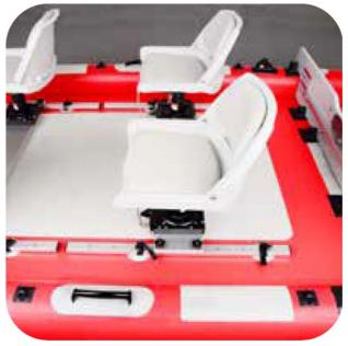
• Attach pedestal to Locking Swivel Seat. Locate swivel seats, 7" pedestals and hardware. Pedestal to seat hardware:  $4 - \frac{1}{4}$ " x  $\frac{1}{2}$ " hex head screws
