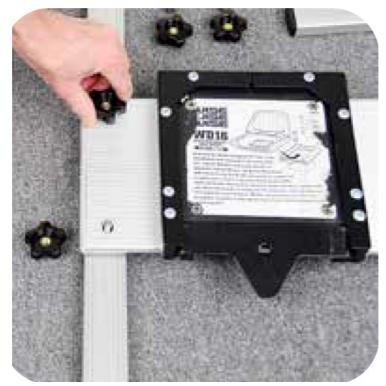
• Place frame on the boat. Frame bars go on top of floor hold down straps. Line up adjustment knobs with hold down straps. Straps go between the knobs so the frame cannot move.
