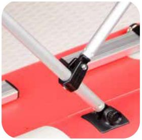
• Use the M6 x 35mm (1 3/8") screw and the knob to secure the rods to the black canopy pads on the boat.
