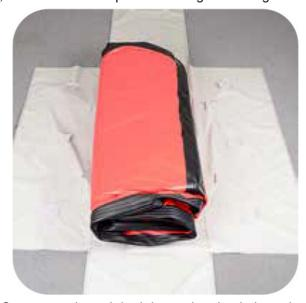
• Secure end flaps with straps. Strap goes through both loops then back through one loop.
