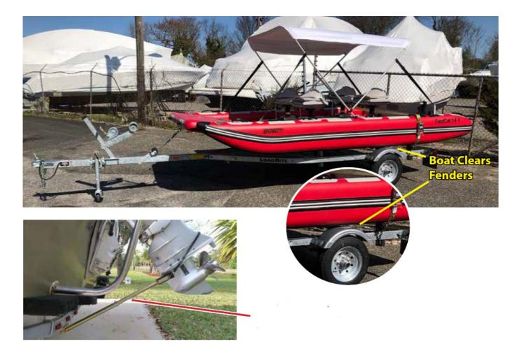
• Transom Saver keeps the motor secured at an angle.
