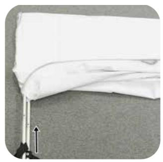
• Place the canopy on the back of the boat. Arrange the bars so the long bar is on top and the short bar underneath.
