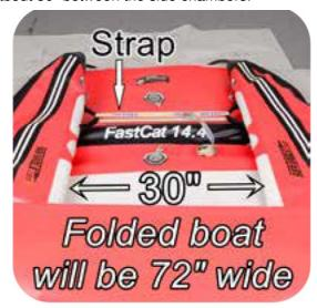
• End caps will be centered on bow handles. At the back of the boat, the side motor mount grommets will be touching the inner motor mount grommets.
