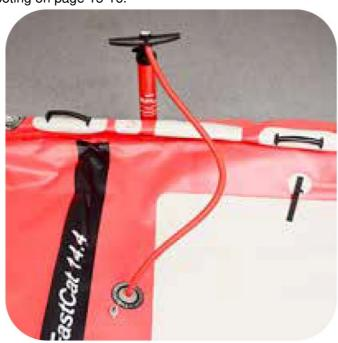
Pressure gauge will not register until chamber begins to get pressurized. Pump until working pressure of between 13-14.5 PSI is reached. Do not exceed 15 PSI (1 bar).
