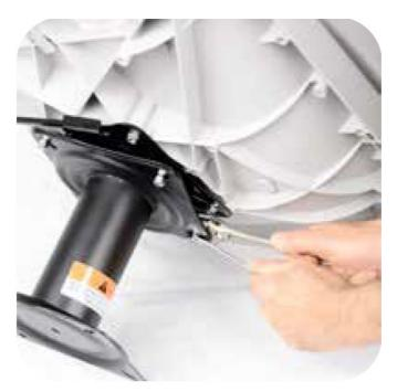
• Slide seat onto seat release. When seat is fully pushed into seat release, the locking mechanism will pop down with a click.
