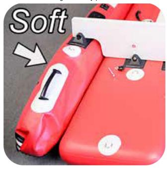
• Insert screws with washer through the side chamber grommets and transom holes. A wrench is recommended for holding the bolt heads while tightening the threaded knob.
