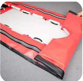
• Once the final fold is reached, the boat will be in position to begin securing the boat bag.
