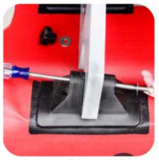
• Pump air into the side chambers to give them enough shape to raise the motor mount grommet near to the transom.
