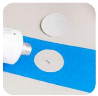
• Apply patch to the boat. Smooth with finger or a smoothing tool such as a spoon, handle of a utility knife, or screwdriver. For best results, heat patch with a hair dryer 10-20 seconds and smooth with tool.
