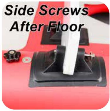
• When all transom screws have been inserted, inflate the sides to working pressure.
