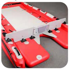
Seat Frame Assembly FastCat14.4 can take up to four seats with pedestals. Seats are installed on alu-minum Seat Frames.
