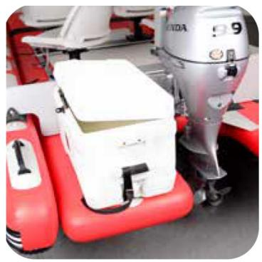
• Run and 8' strap between the D-rings. Place cooler over the strap. Run strap through handle or slot and back under the cooler. Run strap through handle or slot and tighten.
