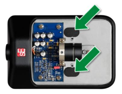
Then use a sharp tool to punch through the underlying protective foil, and mount as desired with screws (not included).
