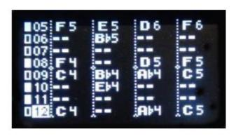
The TRAX editor can sequence up to 64 steps with up to 4 lanes of notes per step. Ideally, this matches the 4 rows of jacks on the panel, which can be assigned in the [SETUP] QB in the pop-up. First a quick break-down of the TRAX sequencer grid. The first column, little rectangles, displays the Note-FX mask cycle.
