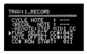
In addition to being able to record notes into the TRAX grid, steps can be modified remotely using MIDI CC's on the TRAX remote MIDI Channel, in a similar way to a normal sequencer module.
