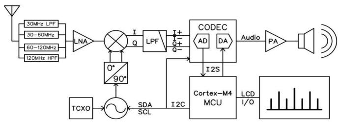
The clock generator Si5351 generates two quadrature square wave signals with variable frequency as excitation, and realizes an ultra-low noise ZIF zero-IF receiver. The IQ signal obtained after mixing is output to the CODEC and collected by the MCU, and the DSP algorithm in the MCU completes the demodulation and display of the signal.
