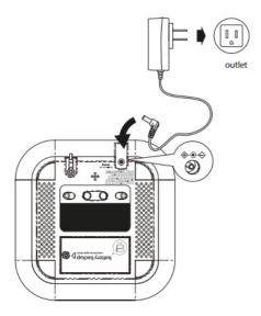
Connect the universal voltage AC adaptor to the DC jack on the bottom panel of the unit.
