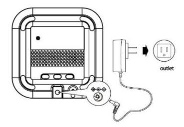
Connect the universal voltage AC adaptor to the DC jack on the bottom panel of the unit. Plug into a wall outlet that is not controlled by a light switch and is within easy reach of the unit.
