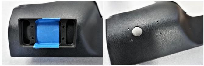
4. Turn the panel over and trim any ribs that would keep the backers from mounting flat against the back side.
