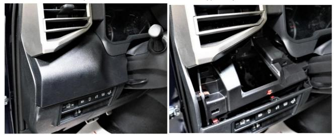
3. Position and secure with tape, your bare keypad mount on the dash trim piece as pictured. Drill a 1/8" pilot hole into the panel using each of your mounts bolt holes as a guide and another pilot hole in the center opening of the bare mount towards the front of the panel. Remove the keypad mount and re-drill the (4) bolt holes with your 5/32" drill bit and use your step drill bit to drill your center hole to 3/4" for the wire harness.
