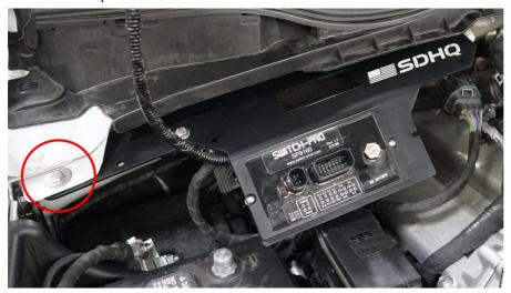
10. Thread and tighten the 15mm nut onto the stud it was removed from in Step 2 or Step 6. Tighten the 10mm PCM nut. Tighten the 1/4" hardware with the fender washer, then the other 1/4" hardware.
