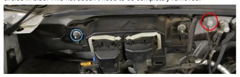
7. Slide the SDHQ Power Module Mount Bracket behind the PCM nut loosened in Step 6. Tighten this nut until the bracket doesn't fall. This will be tightened in a later step.
