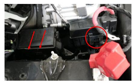
4. Remove the (3) PCM connections. The grey handles are tabbed in place, push in the tab and rotate the handle. Below the PCM connectors are white and black electrical connections, arrowed at below. It may be easier to disconnect these. Remove the plastic panel those are connected to from the plastic cover by pressing the tab down, arrowed at right in blue.
