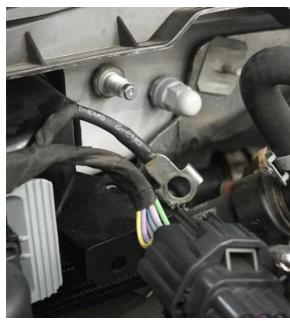
3. If applicable, the fuse boxes clipped to the side of the battery box will need to be moved to allow enough space for removal of the plastic cover. Disconnect the 10mm nut securing the power wire from the fuse box. The cover for this fuse box will need to be opened to access a clip near the battery, circled right. Push in this clip and pull up to disconnect it from the battery box. Repeat this for the (2) clips securing the fuse box closer to the fire wall, arrowed at right.
