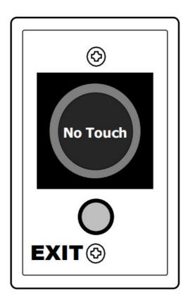
**NOTE:** The SDC 474MU must be mounted to a single-gang electrical back box or plaster ring. All national and local codes must be followed in the installation of the 474MU.
