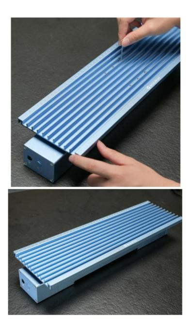
You can adjust it through the two screw holes on the front platform to tighten it when the working platform wobbles too much.
