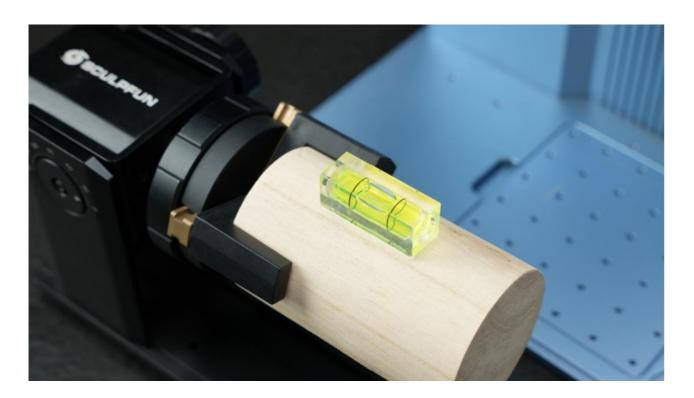
**Step 3: Connection**Use one end of the connection cable to connect the rotary roller, and the other end to connect the accessory interface on the back of the G9 using an adapter cable. After that you can turn on the machine for use.
