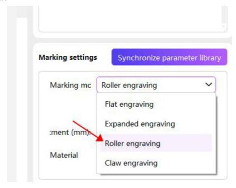
Measure the Diameter of the material in advance (Note That It Is Not The Circumference) and enter it into the software.
