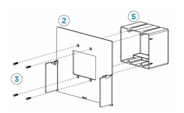
STEP 2: Attach Camera Plate (No. 1, Qty 1) to RCM Wall Plate using 6-32×3/8" pan head Torx screws (No. 4. Qtv 2).
