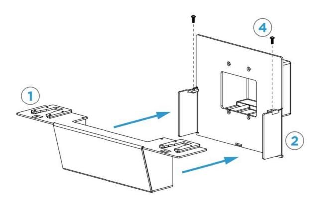
STEP 3: Attached Cisco QuadCam (No. 6, Qty 1) to Camera Plate.
