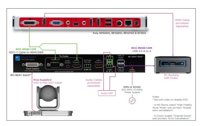
Adding Soft Codec Support to Poly Camera (No Codec, no DSP)
