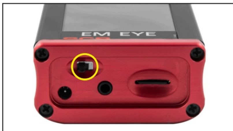
Figure 7. Location of the power switch at the bottom of the EM Eye Meter
