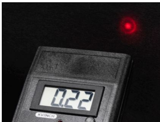
Figure 7. Aligning the two bullseyes emitted by the LED range indicator
