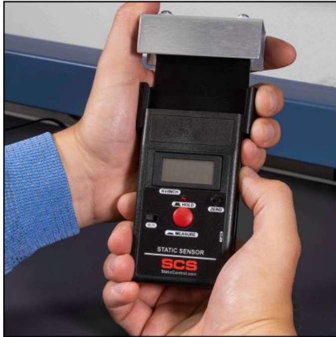
Figure 8. Sliding the Conductive Plate onto the Static Sensor
