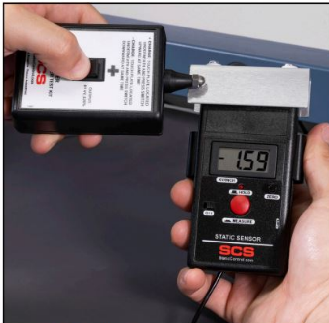
Figure 10. Using the Charger to apply a charge onto the Conductive Plate
