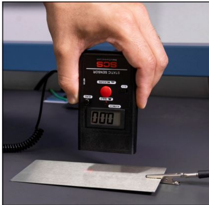
Figure 6. Pointing the Static Sensor to a grounded surface
