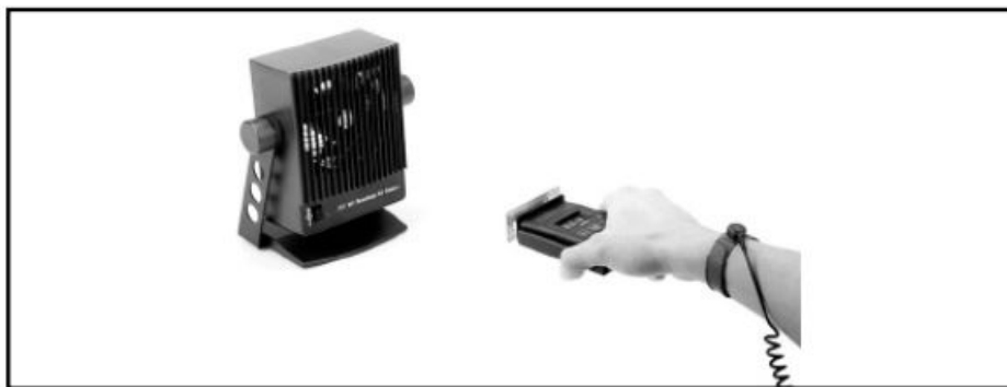
Figure 7. Testing Ionizer Offset Balance.
