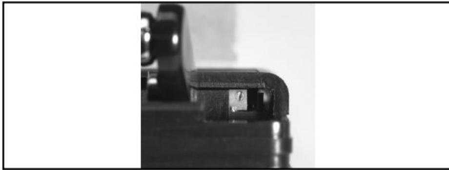
Figure 9. 718 Static Sensor adjustable screw for display.
