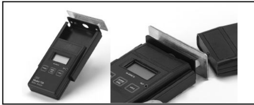
Figure 6. 718 Static Sensor charging plate in use.
