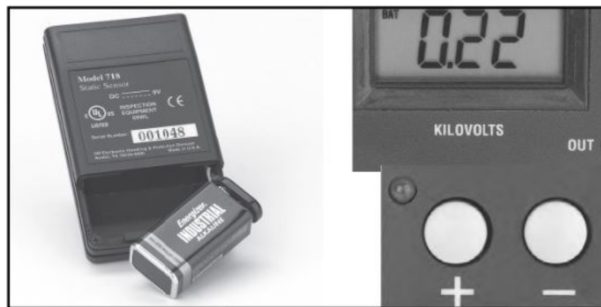
Figure 2. SCS 718 and 718A Battery Replacement and Indicators.
